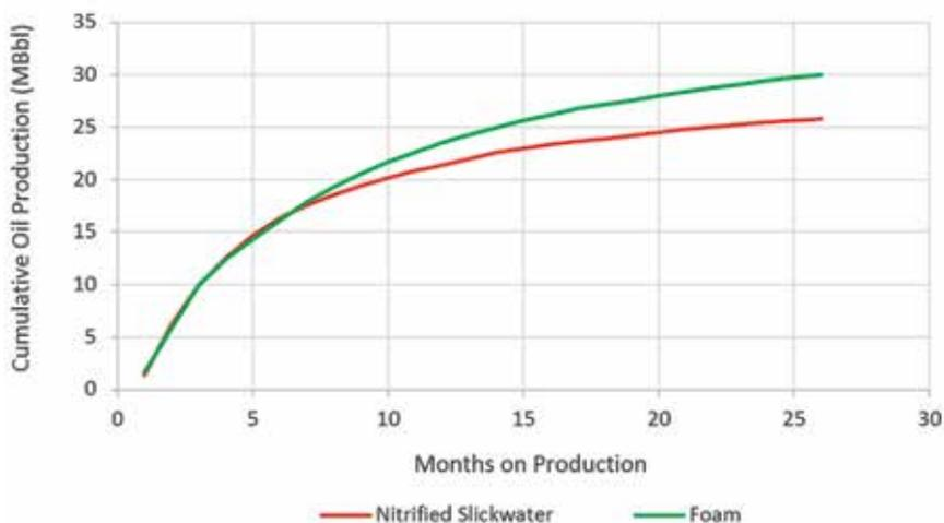
A production curve chart shows the difference in cumulative oil production in the Buck Lake field located in the Cardium formation in western Canada. The slickwater used had a nitrogen content of 12% compared with 58% for the foam treatment. *Graphic courtesy of the University of Texas.*
