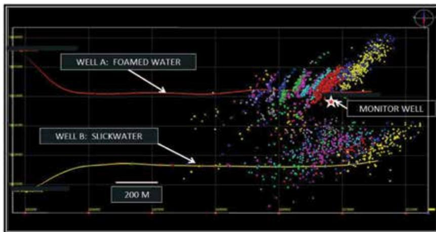
This chart shows the variation in the microcosmic signature of a slickwater and energized foam treatment in two western Canadian wells in which the same tonnage was pumped downhole to the same number of stages. The data shows the relative uniformity of seismic events with the foamed fracture, compared with the more scattered events in the slickwater fracture. *Source: Paper SPE 166268.*
