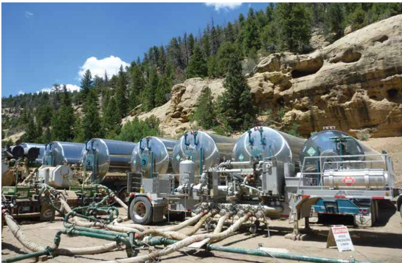
As an alternative to slickwater, an energized fluid containing carbon dioxide is pumped into a horizontal well during fracturing operations in the Mancos shale play amid the rugged terrain of Grand County, Utah. *Photo courtesy of Ferus.*
