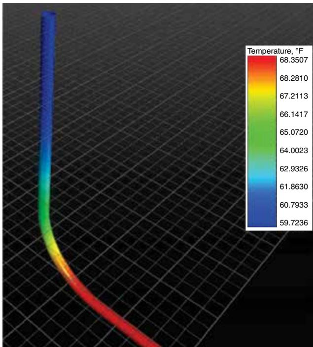
The software, ERAC-3D, developed by the University of Texas, combines fracture, wellbore, and well productivity models for energized foams and fluids, as well as all other conventional fluids such as slickwater and gels. *Image courtesy of the University of Texas.*
